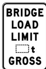
Bridge load limit (gross mass) sign
