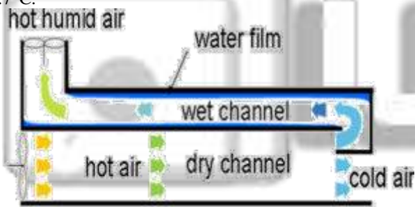
Fig. 2: Schematic of Regenerative Evaporative Cooler.
