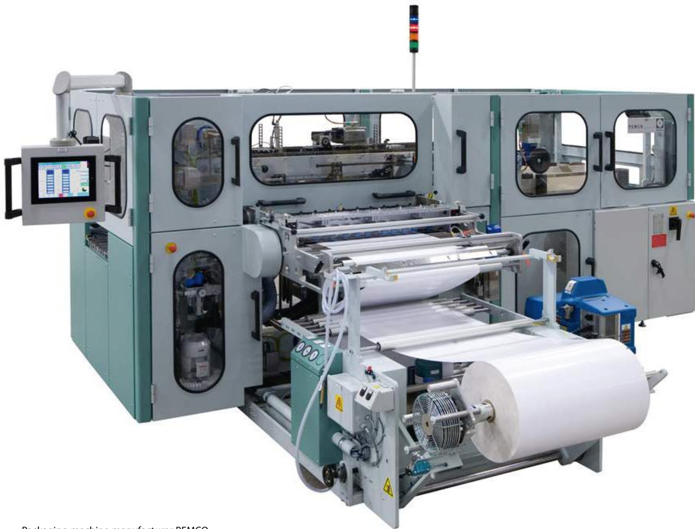
Packaging machine manufacturer PEMCO relies on PROFIdrive: flexible giant wrapping machines for layered or laminated paper and polypropylene film
