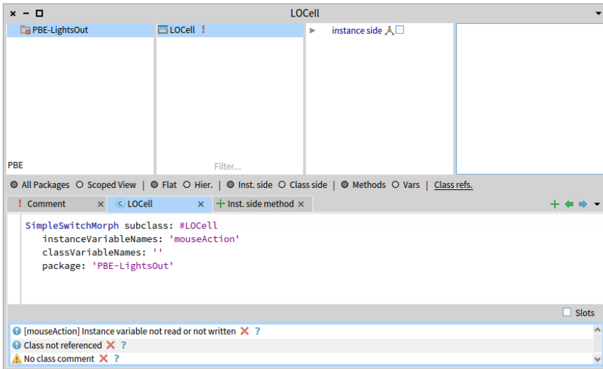
Figure 6-5 The newly-created class LOCell.
