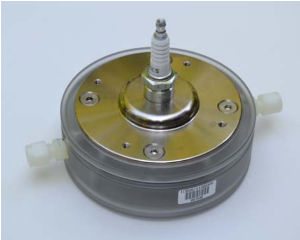
Model SG-101BM trigatron (electrically triggered) switch for moderate HV applications: 10–40 kV, 100 kA, <35 nH
