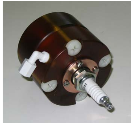
Model SG-104B demountable mini-trigatron switch: 5–40 kV, 65 kA, ≈35 nH
