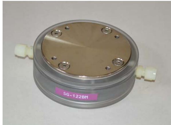
Model SG-102BM passive (self-breakdown) switch: 20–40 kV, 85 kA, <35 nH
