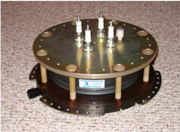
Model SG-151M multichannel trigatron switch for extreme current, large charge-transfer applications: 10–40 kV, 400 kA, 8 C, <30 nH
