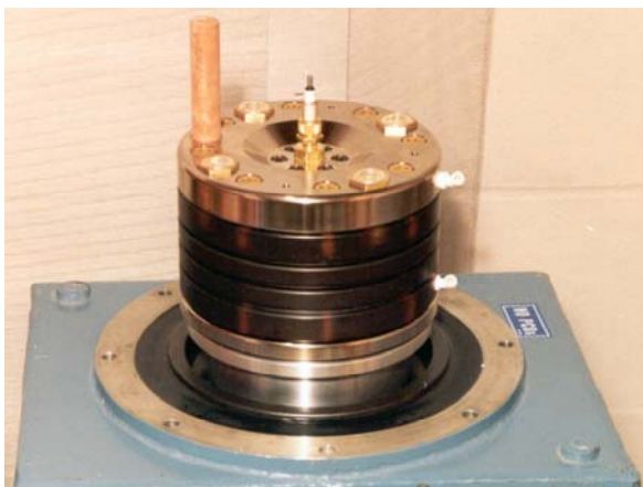
Model SG-182 trigatron switch for direct mounting on Scyllac-style capacitors: 15–60 kV, 250 kA, 1 C, 27 nH (companion shield canister not shown)
