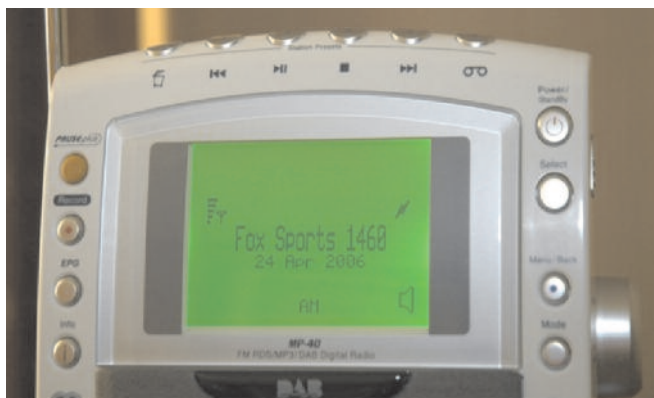
Figure 5.4: Screen-shot of DRM receiver in AM mode displaying AM service name
