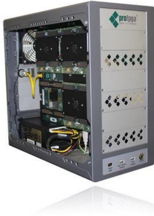
Figure 8.4: Optional case for FPGA
