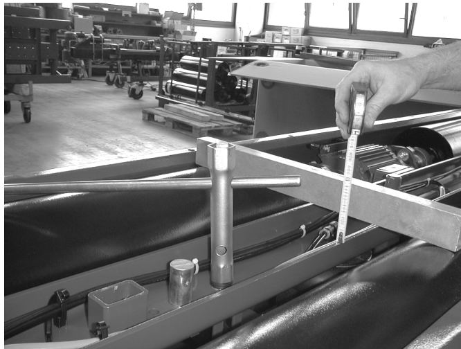
Setting of the lift beam
